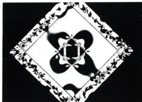
↑ Phot. 2 (b) Isocromatic Fringes of Photoelasticity for \diamond -shaped Bracings in Square Opening Subjected to Shear Force
